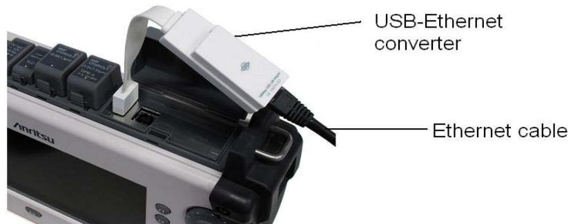
Figure 14-2: Ethernet Cable Connection
