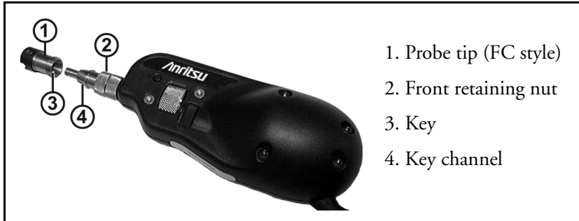
Figure 11-4: Attaching a Probe Tip
