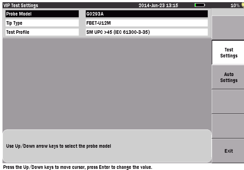
Figure 11-9: VIP Test Settings Screen
